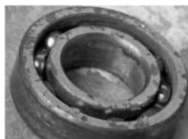
Figure 2. A Bearing fault caused by corrosion
