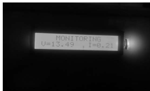
Fig 4.4 Testing voltage and current sensors with load
